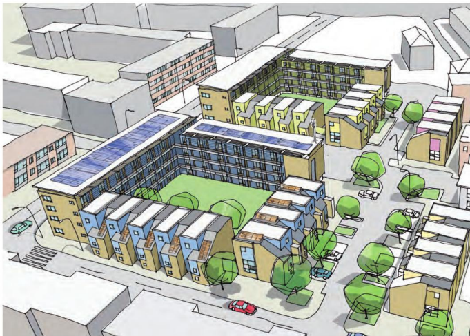
11.14 Future-proofing the scheme with photovoltaics.
